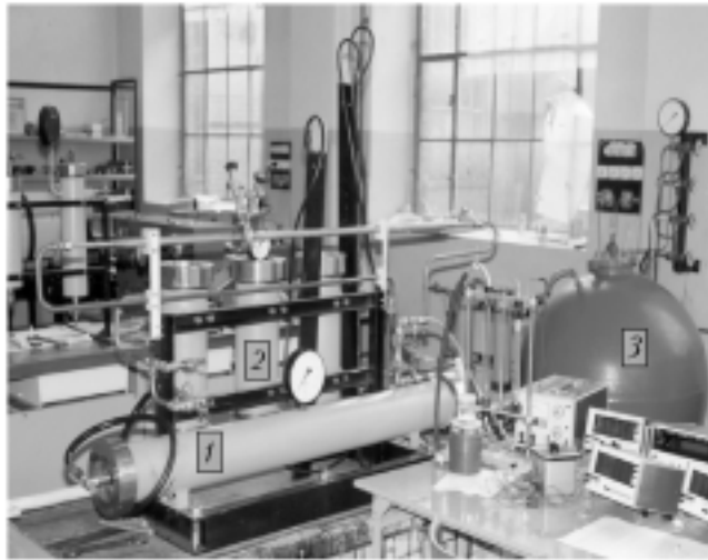
Fig. 1. A view of a rig for investigation of convective processes under high-pressure conditions (research chamber positioned horizontally): 1) research chamber; 2) pressure tanks; 3) storage tank.
